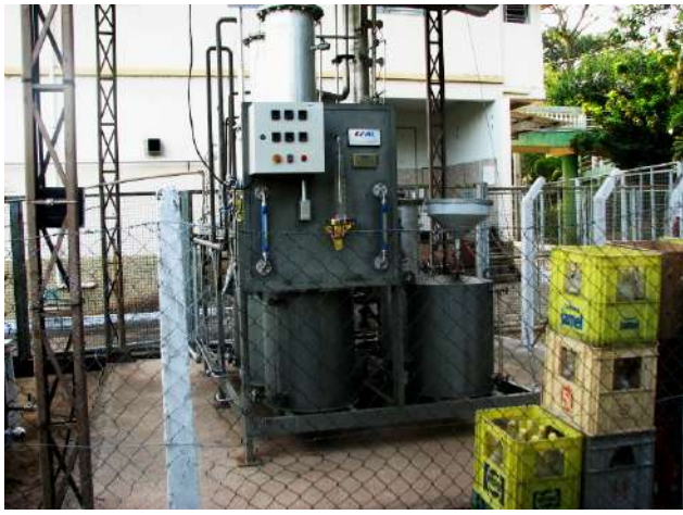
Figure 17: Inconfidentes Campus alcohol distiller.
