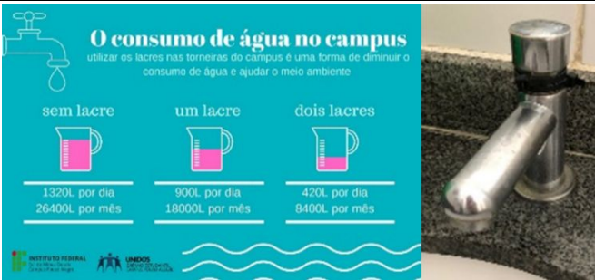
Figure 7: Campus Pouso Alegre tap with cable ties.
