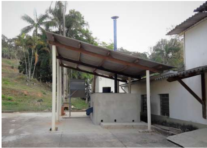
Figure 13: Inconfidentes Campus fixed box coffee dryer (static dryer).
