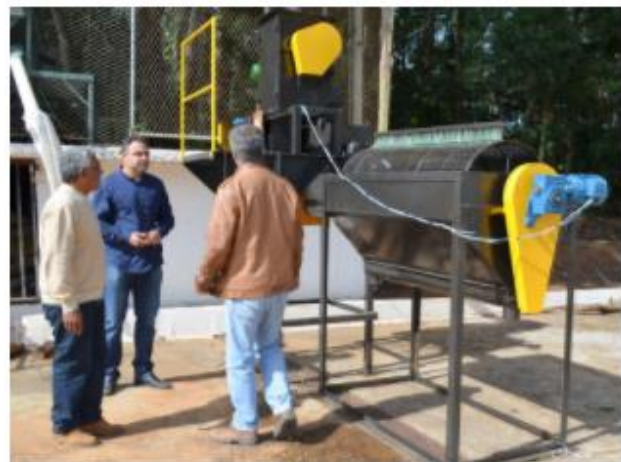
Figura 4 Campus Machado - Coffee peeling machine
