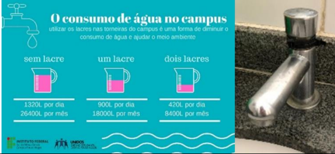
Figure 7: Campus Pouso Alegre tap with cable ties.
